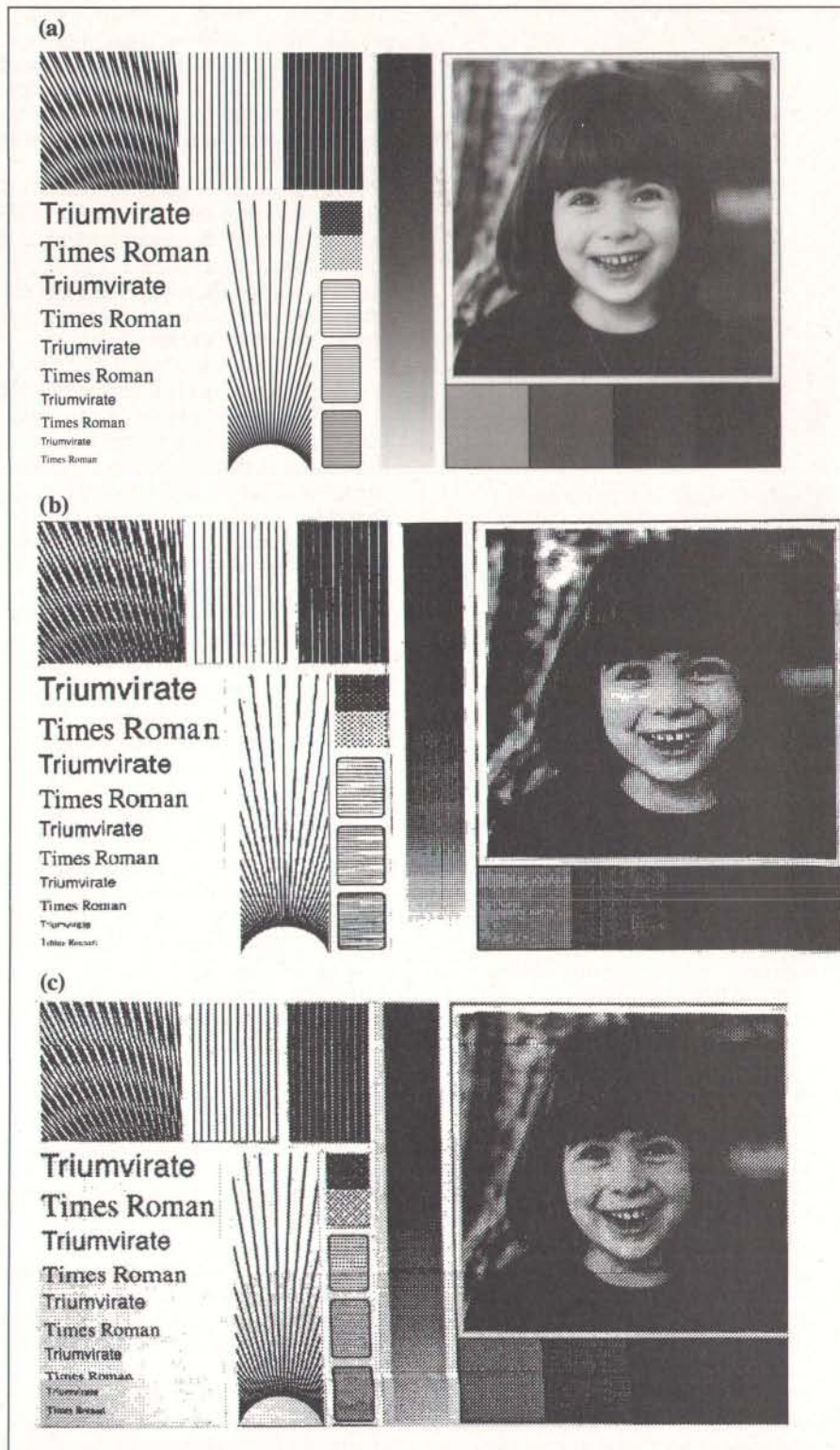
Figure 1: The BYTE scanner template (a) and the best results we could obtain for each scanner tested. We performed all scans at medium brightness. (b) The Complete Hand Scanner/400 at 300 dpi with spiral dithering. (c) The HS-3000 at 300 dpi with middle-dot translation. (d) The Niscan at 200 dpi with gray spiral. (e) The ScanMan at 300 dpi with small-dot translation. (f) The SkyScan at 200 dpi with halftone setting. Missing is the GS-2000 Plus, which produced only a partial image at its best setting.
